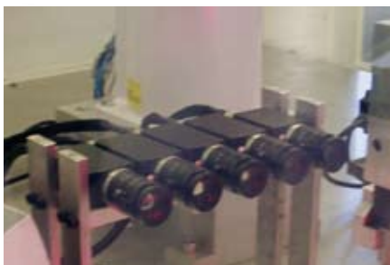
CDC cameras for dimensional check of load pin
